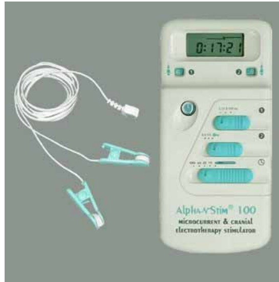
Figure 1: The Alpha-Stim 100 Cranial Electrotherapy Stimulator with ear clips. Study settings were at 0.5 Hz for 1 Hr. Sham ear clips did not pass current.
